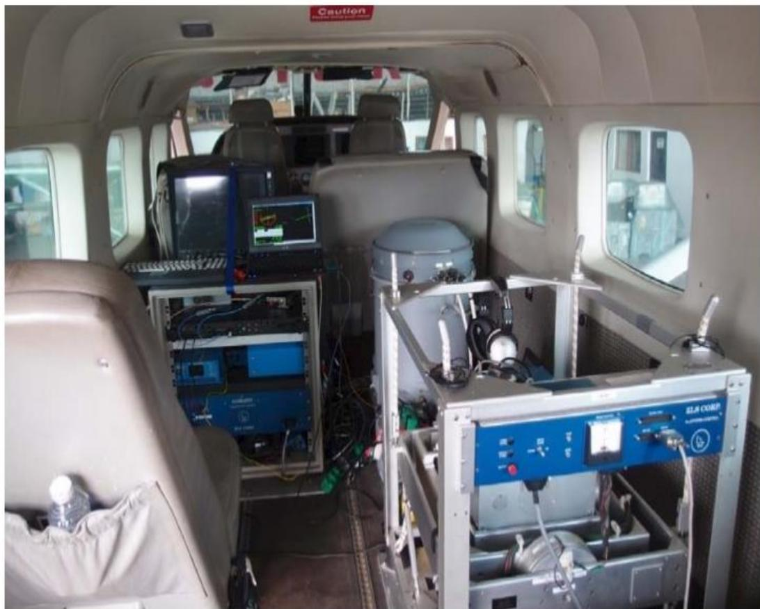
Figure 5. Cabin layout in the Cessna Caravan aircraft. To the right, the LCR gravimeter and behind it the Chekan meter
