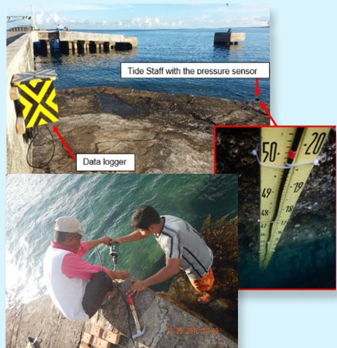
Figure 29. Establishment of temporary tide gauge
