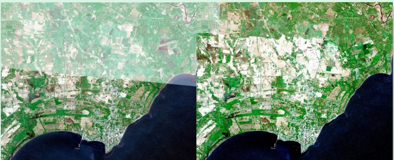
Figure 10. Colors are matched between multiple scenes (left) to create a seamless mosaic (right) of the area. Images are usually cut along identifiable features (e.g., roads, paddies) to make seams less prominent.
