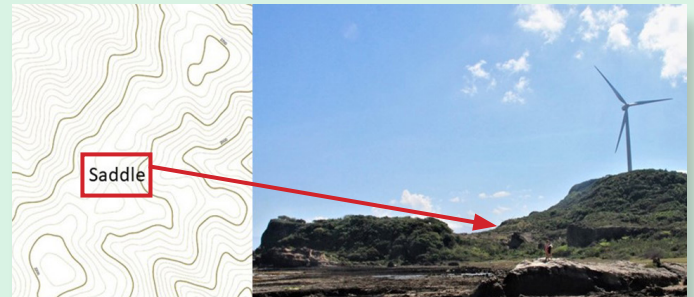
Figure 16. A saddle is a low point between two hilltops or peaks.
