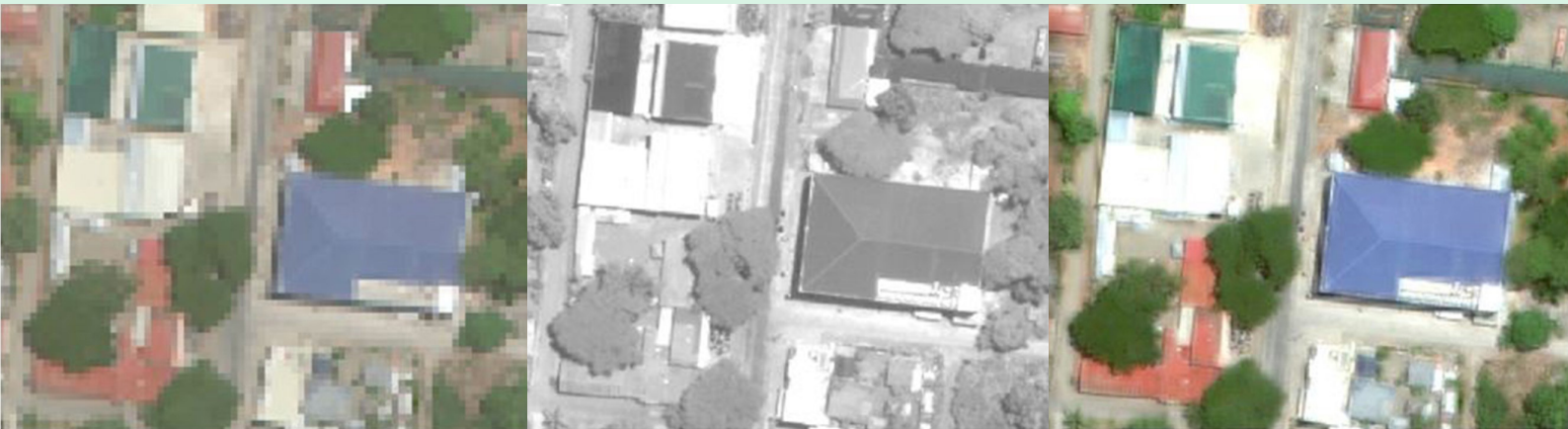
Figure 8. A multispectral image has a lower image resolution (left) compared to a panchromatic image of the same area (middle). In this example, the multispectral image has a spatial resolution of two meters while the panchromatic image has a spatial resolution of 30 centimeters. The images are processed against each other to create a pansharpened image: that is, a multispectral image with a spatial resolution equal to that of the panchromatic image (right).
