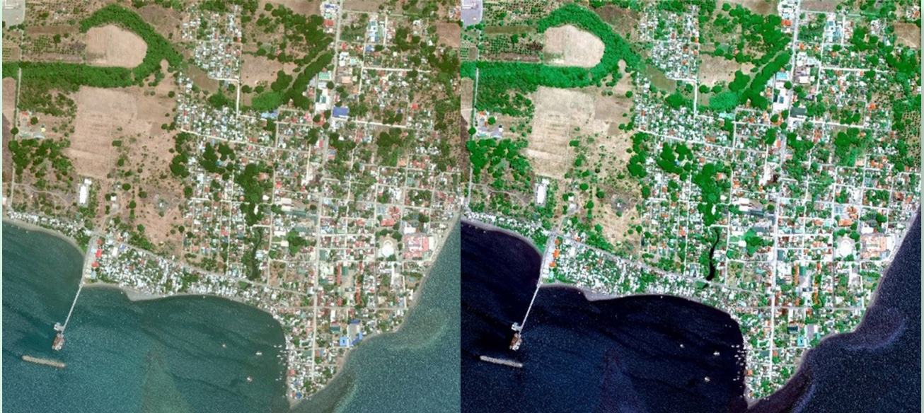
Figure 9. The figures show natural color processing applied over a scene. The unprocessed image (left) returns darker greens over vegetated areas, whereas the processed image (right) shows vegetation closer to their appearance in ideal lighting conditions.
