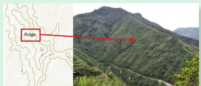
Figure 18. A ridge is located on a high ground which usually connects peaks or hilltops.
