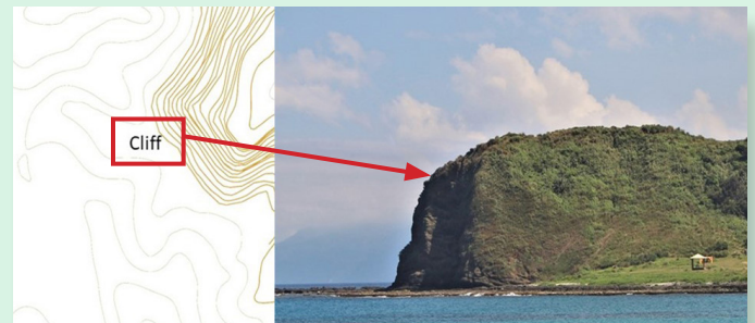
Figure 17. A cliff is a vertical or near vertical ground feature. On a topographic map, cliffs are represented by very close contour lines and sometimes they appear as one line. However, some cliffs may not appear on a topographic map depending on the scale of the map.
