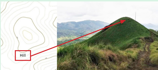
Figure 13. Like a volcano, a hill is composed of contour lines forming concentric circles. The smallest circle indicates the peak of the hill.
