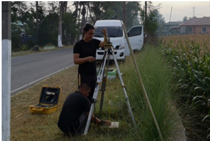
Figure 3. NAMRIA Geodesy Division personnel measuring the antenna height of the GNSS setup in Isabela
