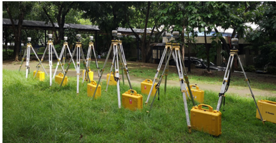
Figure 4. TRIMBLE R10 GNSS receivers tested before the fieldwork
