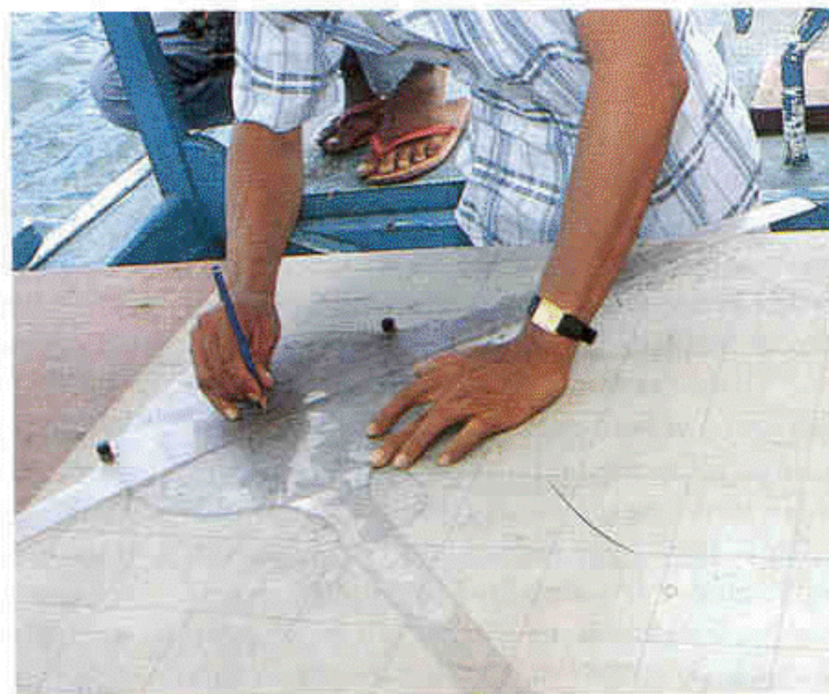
Conventional plotting of a three-point fix using a three-arm protractor
