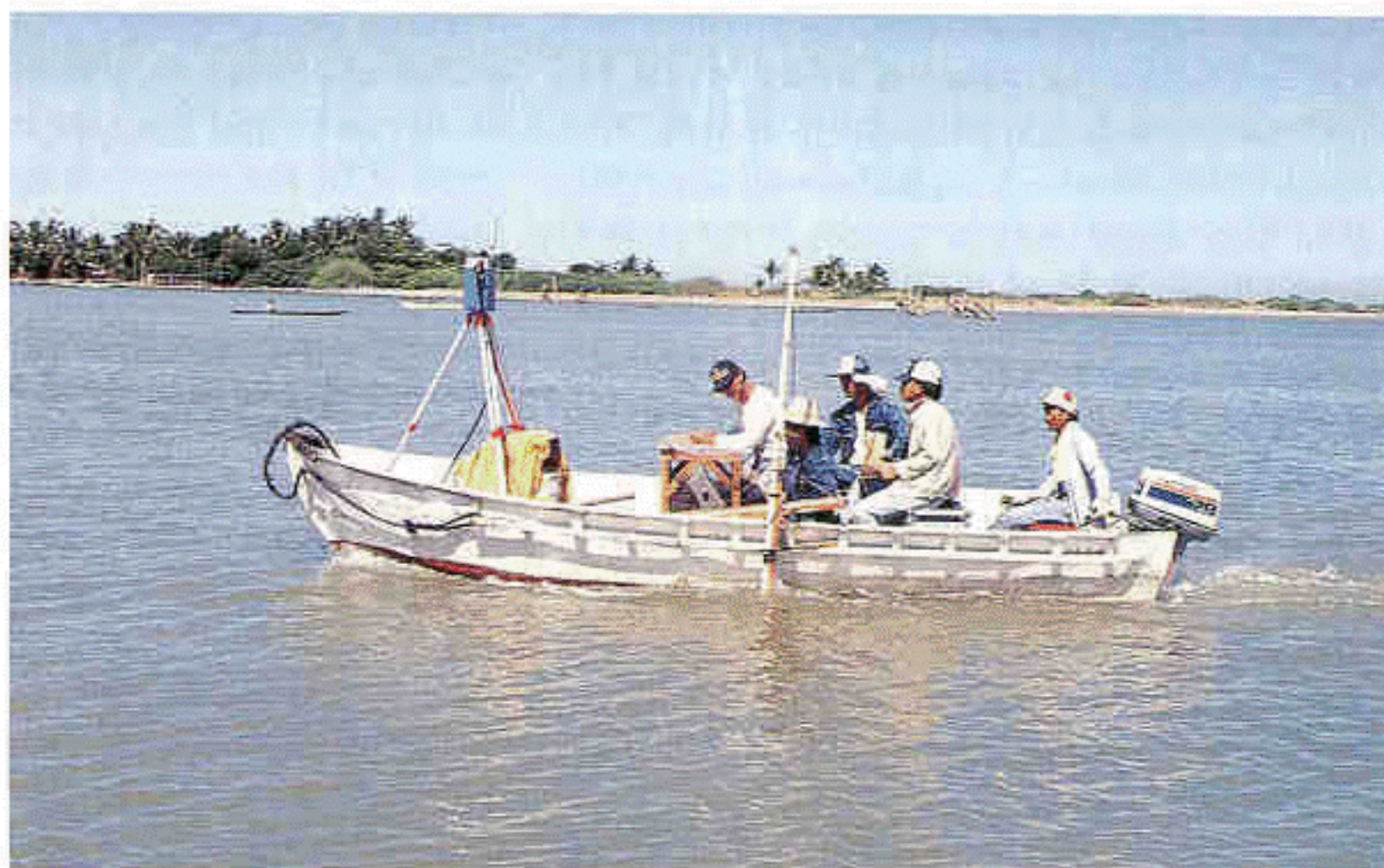
Depth measurements using echo sounder and skiff with outboard motor
