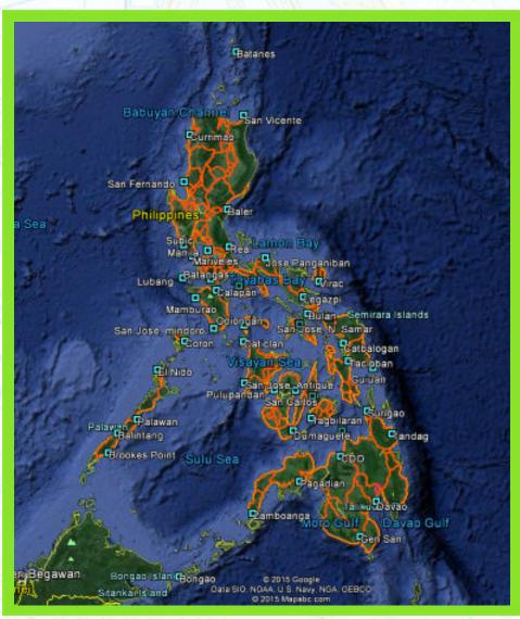
Overlaid on Google-Earth satellite image, map shows the 47 tide stations (in blue boxes) located in strategic ports of the country which were connected to the level network (in orange lines) to give mean sea level elevation to the BMs
