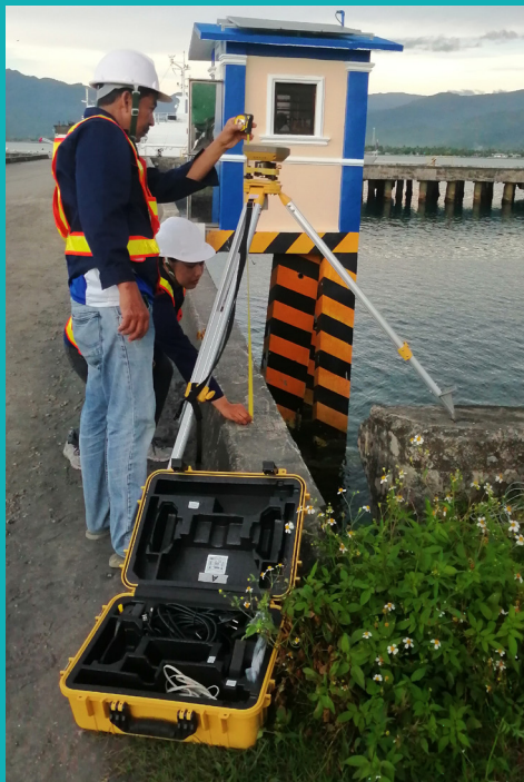
NAMRIA oceanographers conduct tidal leveling and GNSS observation of tide gauge benchmarks.
