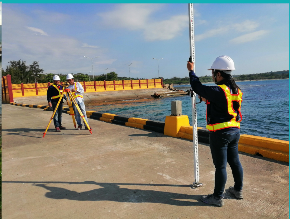
NAMRIA oceanographers conduct tidal leveling and GNSS observation of tide gauge benchmarks.
